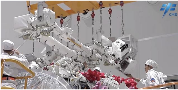
Figure 9. Install the EMM outside the Wentian's cabin.
